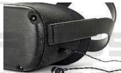
Figure 6: Head Mounted Display of Oculus Quest and its features.
