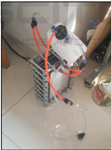
Figure 3: Prototype HHO generator engine.
