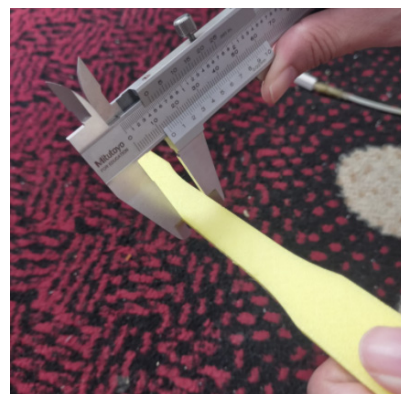
Figure 10: The process of measuring the PETG tensile test specimen from a 3D printer.
