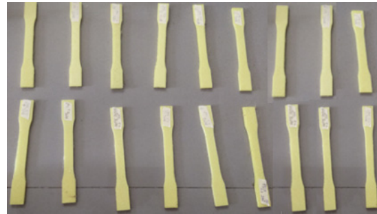
Figure 9: Tensile test specimen results with PETG filament from a 3D printer.
