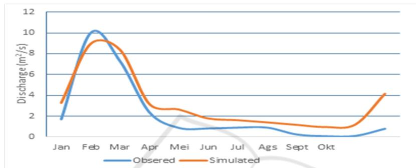
Figure 5: Graph of the relationship between the measurement discharge and the calibrated model discharge.
