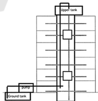
Figure 3: Down Feed System With Spill Back Tank.
