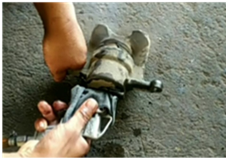
Figure 4: Releasing the brake caliper piston with an air-gun.
