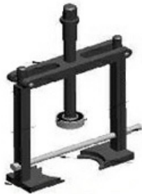
Figure 2: The caliper piston remover tool designed by Setia A.
