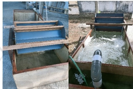
Figure 4: a. Water wheel installation in an open channel (left) b. Rig test to simulate hydraulic behaviour of waterwheel in open channel system. (right).
