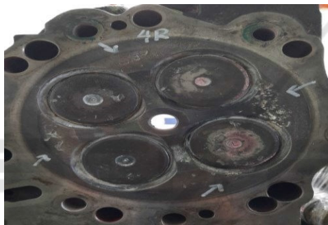
Figure 10: Erosion on cylinder head.
