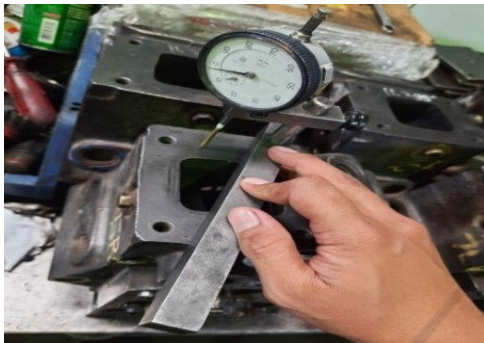
Figure 7: Pitting measurement on cylinder head.
