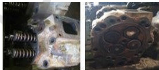
Figure 2: Corrosion on cylinder head.
