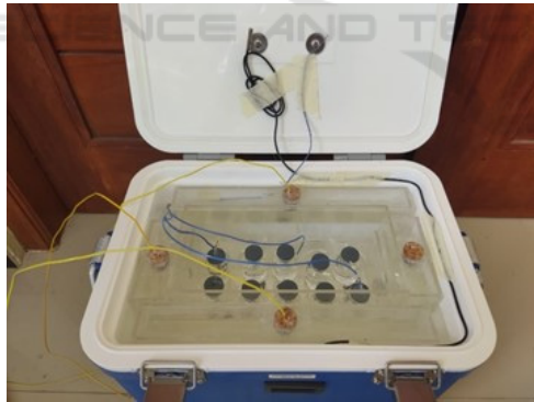
Figure 3: The cooler box completed with bio-Nano PCM containers and vaccine bottle holder.
