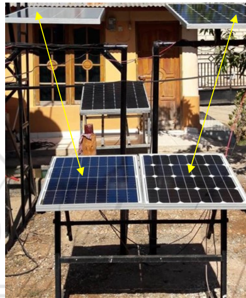
Figure 3: Monocrystalline (right) and polycrystalline (left) solar panels.
