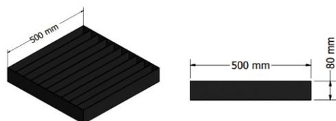
Figure 1: Three Dimensional Model of Solar Collector.
