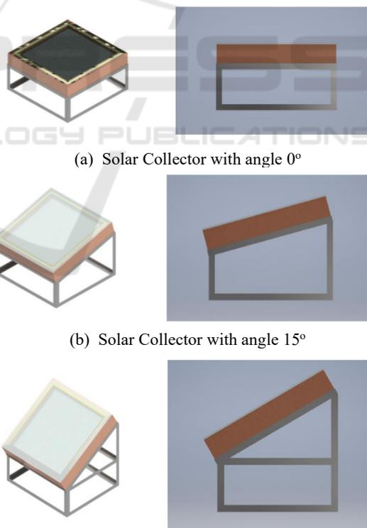
Figure 3: Angle Variation of Solar Collector.
