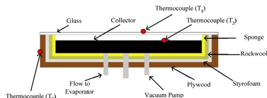
Figure 2: Inside Part of Solar Collector.
