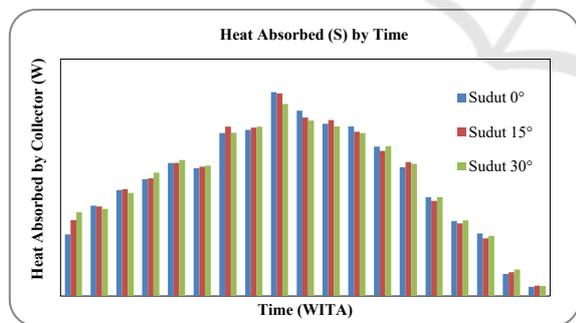
Figure 5: Heat absorbed by Collector.
