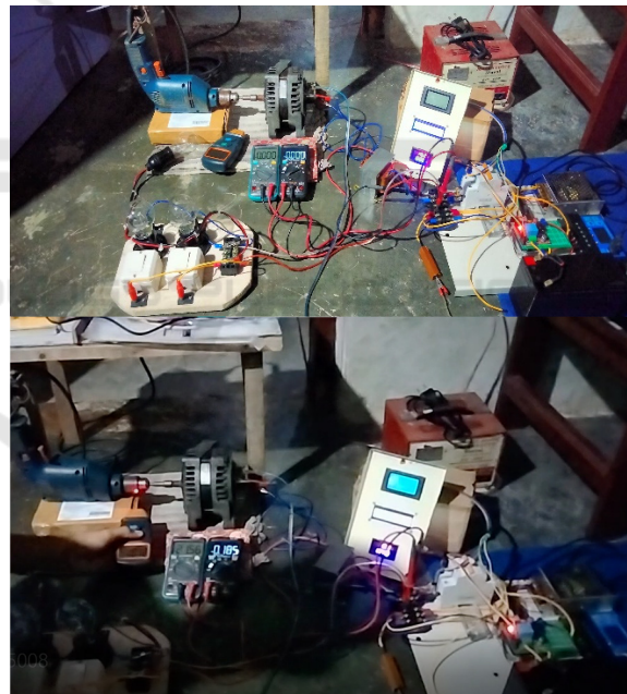
Figure 5: Excitation System Circuit Testing.
