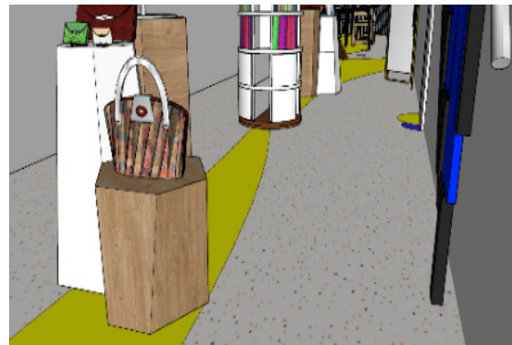
Figure 24: Wayfinding with terrazzo and yellow epoxy as the floor materials.
