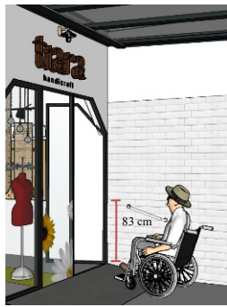
Figure 15: Grab bar at the main entrance.
