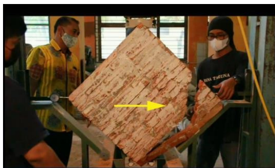
Figure 13: Ordinary brick crack pattern.
