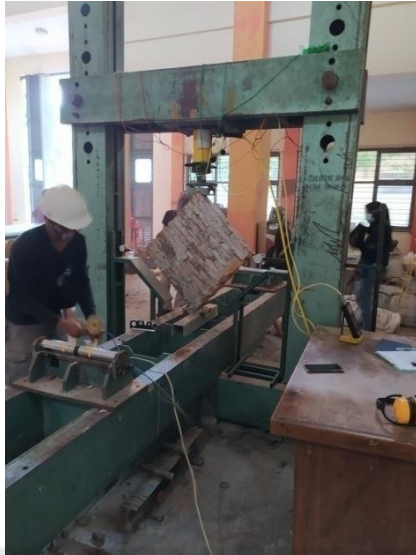
Figure 10: Diagonal shear strength test.
