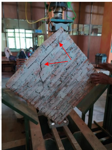
Figure 12: Ordinary brick crack pattern.
