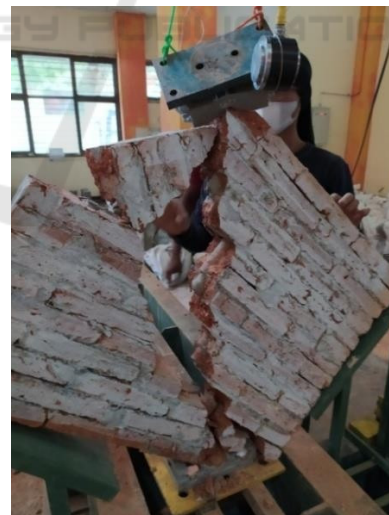
Figure 15: PLB brick crack pattern.
