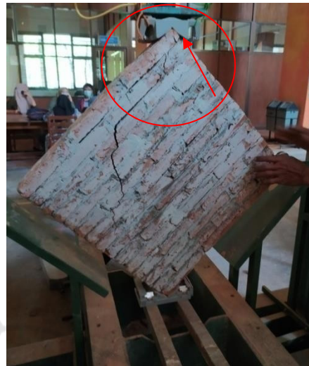
Figure 14: The placement of the corners is not perfect.
