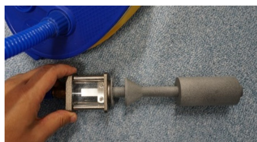
Figure 2: The air pump (in blue), a reed-type sound source (left) and a vocal-tract model (right).
