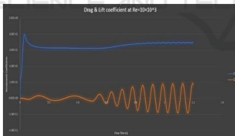
Figure 9: Variation of the coefficient of drag and lift in the case of D=50\text{MM} .
