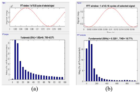
Figure 6: The spectral distribution of the network voltage and current. (with filter)
