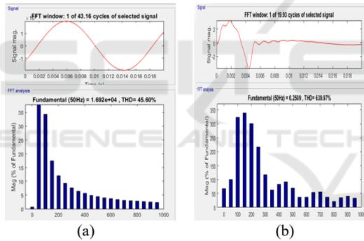
Figure 5: The spectral distribution of the network voltage and current. (without filter)
