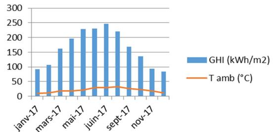
Figure 4: Global solar radiation in (KWh /m<sup>2</sup>), at 31° angle and ambient temperature
