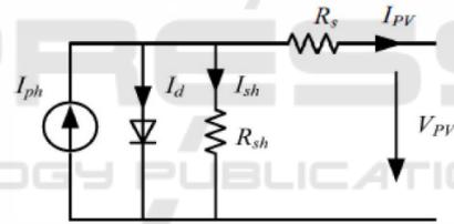
Figure 2: A PV cell equivalent circuit
