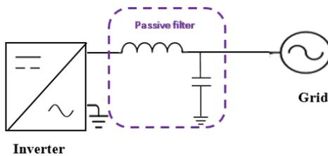
Figure 3: Diagram of a parallel passive filter
