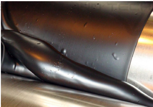
Figure 2: Rubber compound with traces of foreign inclusions.
