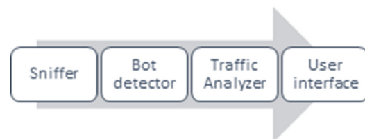
Figure 3: An augmented model of distributed denial of service attack detection system.
