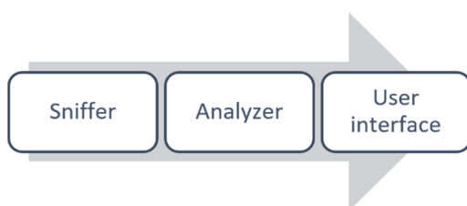
Figure 2: Distributed Denial of Service attack detection system model.
