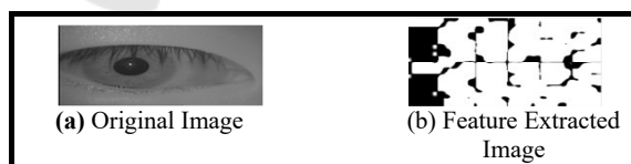
Figure 9: Representation of an iris image to resulting feature image.
