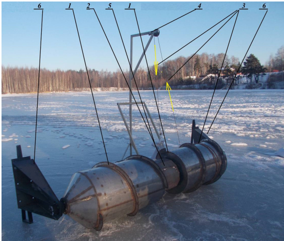
Figure 6: Test bench for determining of the relationship between the generated sound level and the deformation force magnitude of the basic cylinder.
