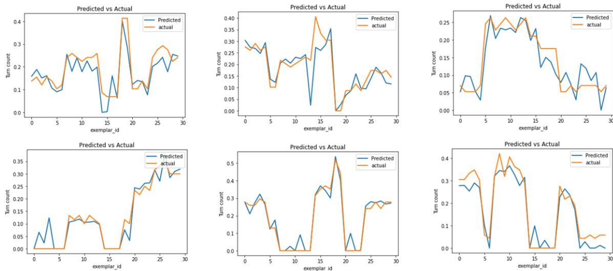
Figure 5: Actual vs. predicted turning movement counts for six different movements using a waveform model. The y-axis represents particular movements; the x-axis represents random exemplars of the test set.
