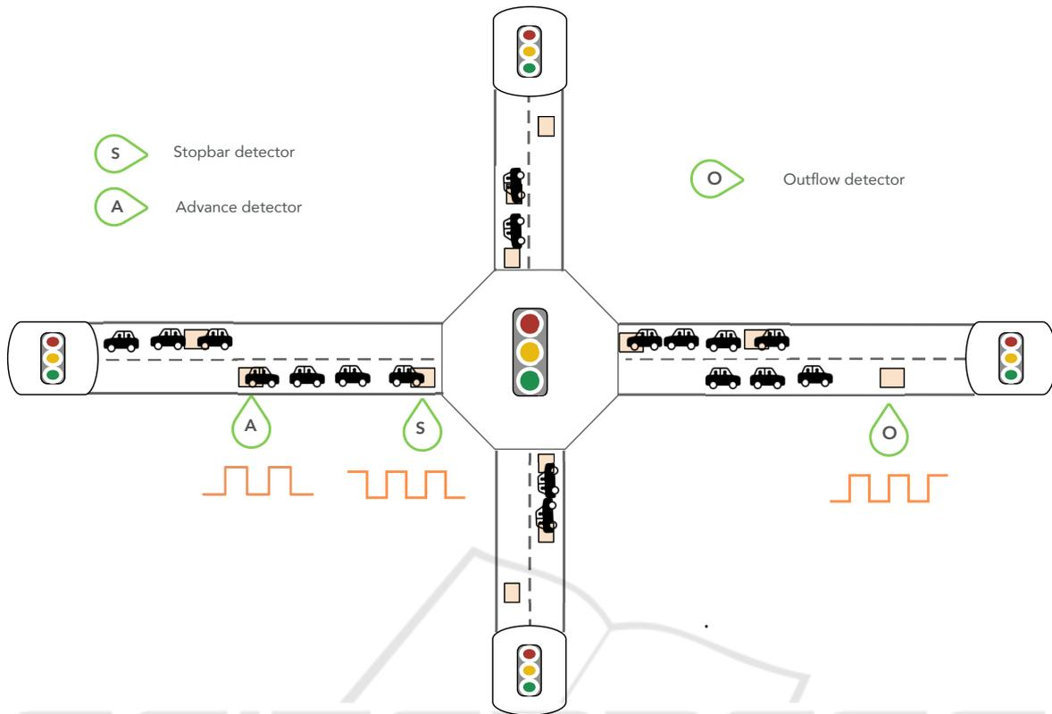
Figure 1: Diagram showing a typical intersection. Arrival/departure waveforms are observed at stop bar (S) and advance (A) detectors.
