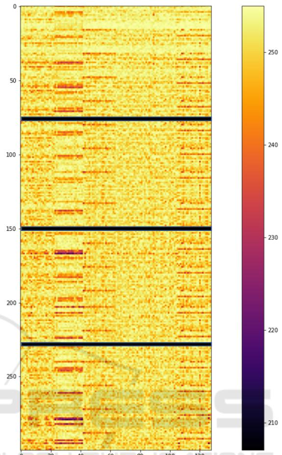
Figure 10: Plot showing heat map of weights connecting input layer and first hidden layer. The horizontal black bar separates the four directions. The ordering of detector waveforms along the y-axis is as follows: east, west, north, and south.
