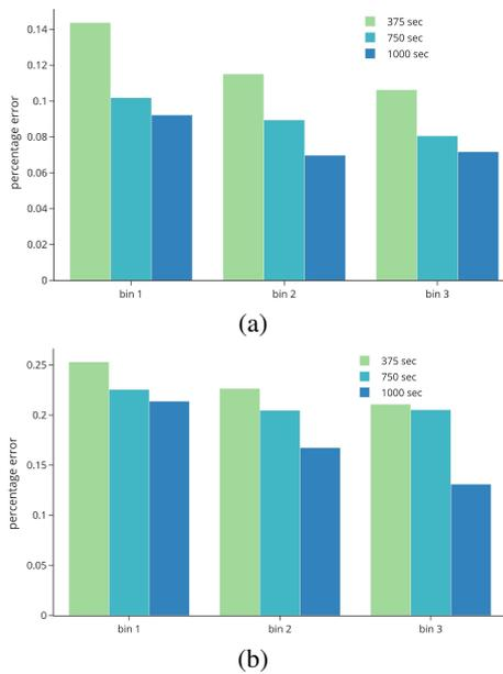
Figure 8: Plot showing percentage error for comparing different prediction windows. This plot suggests that accuracy increases when predicting for a larger window size: (a) eastbound through; (b) southbound through.
