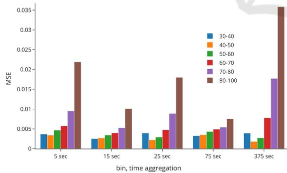
Figure 6: Plot showing MSE for eastbound through traffic for different bins, comparing different waveform aggregation levels.
