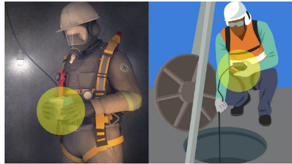
Figure 1: Gas measurement by portable meters: measurement performed by the worker himself (left) and measurement performed by the watchman (right). Source: Author, adapted from (Vale, 2015).
