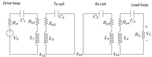
Figure 5: Lumped equivalent circuit of a four coils system.
