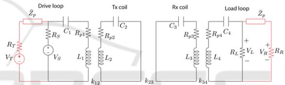
Figure 6: WPT – PLC system characterized by power and data having the same access point.
