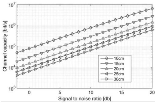
Figure 4: Channel capacity versus distance.
