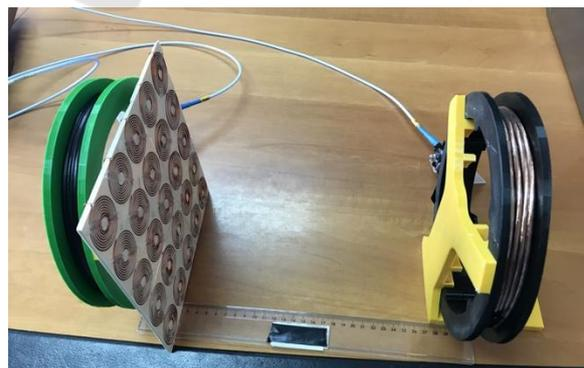
Figure 12: Wireless Power Transfer system with metamaterial slab.
