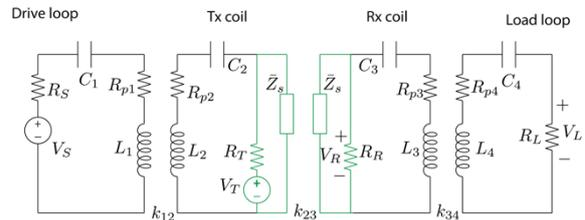
Figure 7: WPT – PLC system system characterized by power and data having different access points.
