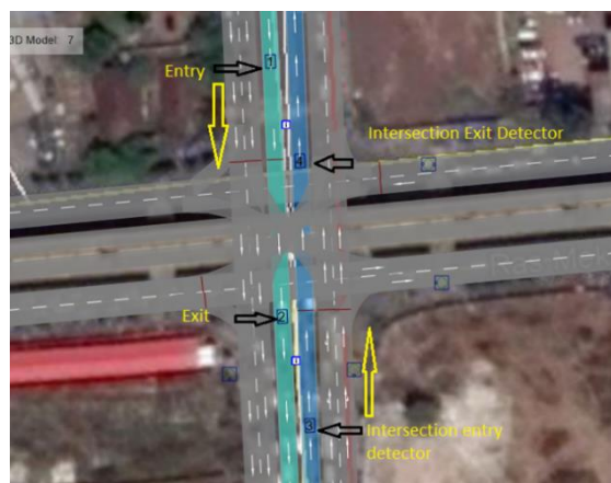
Figure 6: Signal and detector coordination in VISSIM.
