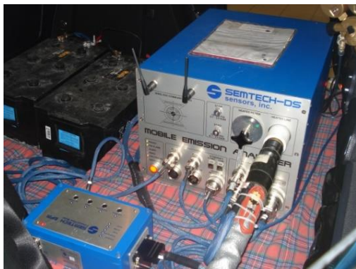
Figure 3: Exhaust emission measurement device Semtech-DS with auxiliary components.
