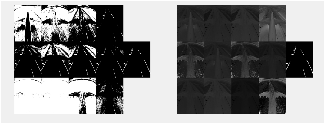
Figure 4: Example of Binary (left) and Distance (right) maps for fin camera images. First line: \Delta E^*_{ab} , \Delta E_{AB} , \Delta E_B , \Delta E^*_{00} . Second line: \Delta E_{LCH} , \Delta C_{LCH} , \Delta E_{CH} , \Delta E^*_{CMC} , ground truth. Third line: \Delta E_{CbCr} , \Delta E_{Cb} , \Delta E_{IQ} , \Delta E_H (HSV/HSL).
