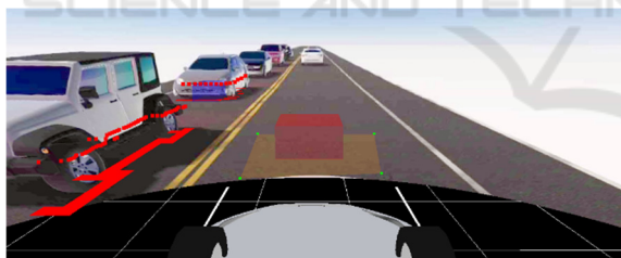
Figure 4: False positive detected object (red) in front of the ego vehicle enclosed by a clicked polygon (green points, orange area).
