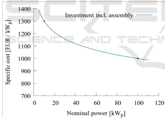
Figure 1: Dynamic cost function (1), with data points (10kW<sub>p</sub> | 1,300EUR/kW<sub>p</sub>) and (100kW<sub>p</sub> | 1,000EUR/kW<sub>p</sub>).
