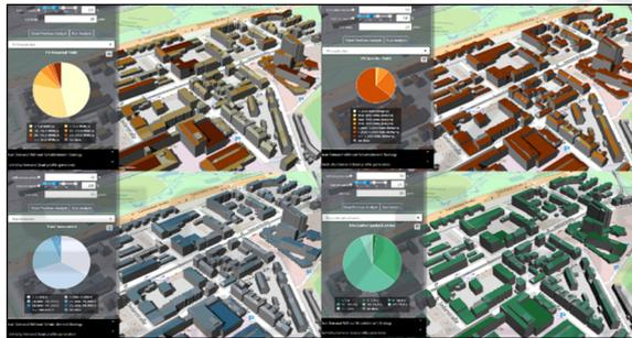
Figure 3: Visualization of PV potentials and economics; Top left: PV yield in MWh/a; Top right: LCOE in EURct/kWh; Bottom left: total investment in EUR; Bottom right: discounted payback period in years.
