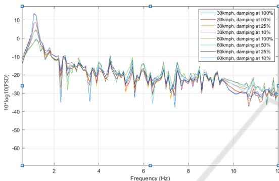
Figure 5: Power spectral densities for sprung mass acceleration of different damping coefficients with different velocities.
