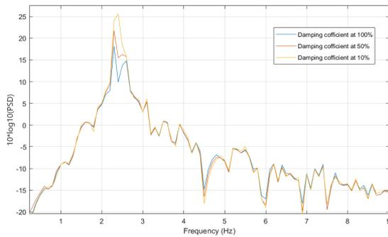
Figure 4: Power spectral densities for sprung mass acceleration of different damping coefficients.
