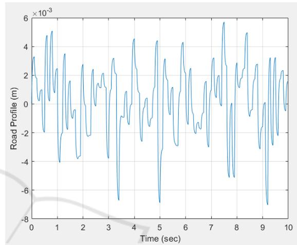
Figure 3: Road surface (class C, velocity 80 kmph).
