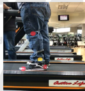
Figure 4: Depicts the tracking measures performed with the foot drop patient using the treadmill.
