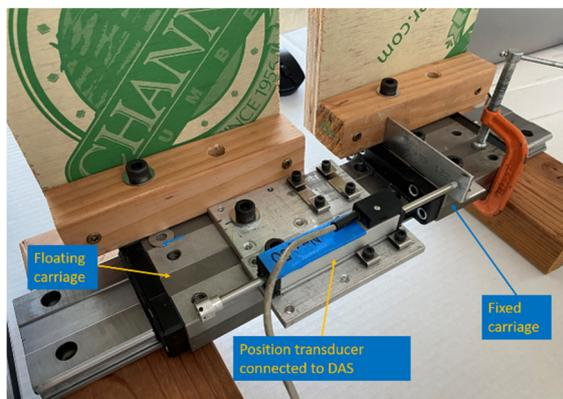
Figure 4: Reference position transducer to monitor relative displacement.
