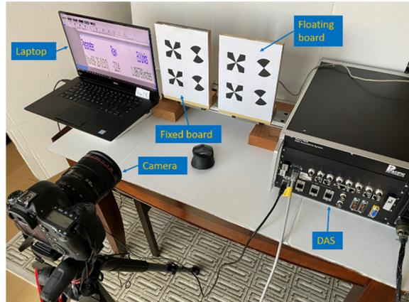
Figure 2: Front view of experimental setup.
