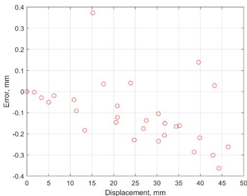
Figure 12: Error of target's center estimation with respect to the reference position transducer.
