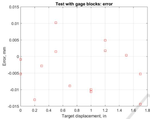
Figure 7: Error of position transducer with respect to gage blocks.
