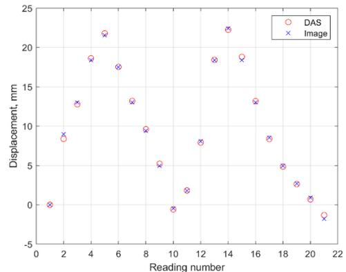
Figure 16: Comparison of the displacement measured from images to that of the reference position transducer.
