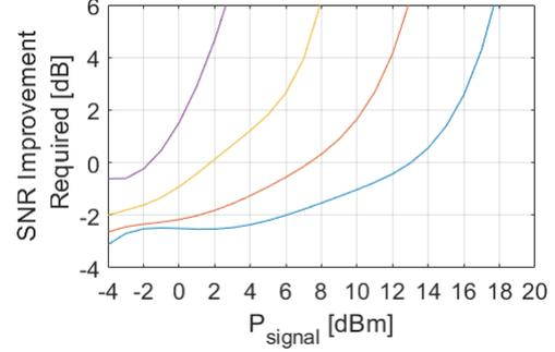
Figure 7: SNR improvement required as a function of the NRZ signal mean optical power, for different carrier mean optical power levels: 0 dBm (blue), -5 dBm (red), -10 dBm (yellow) and -15 dBm (purple).
