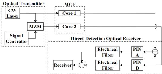
Figure 1: Equivalent model of the MCF-based transmission scheme with DD and SSBI removal.
