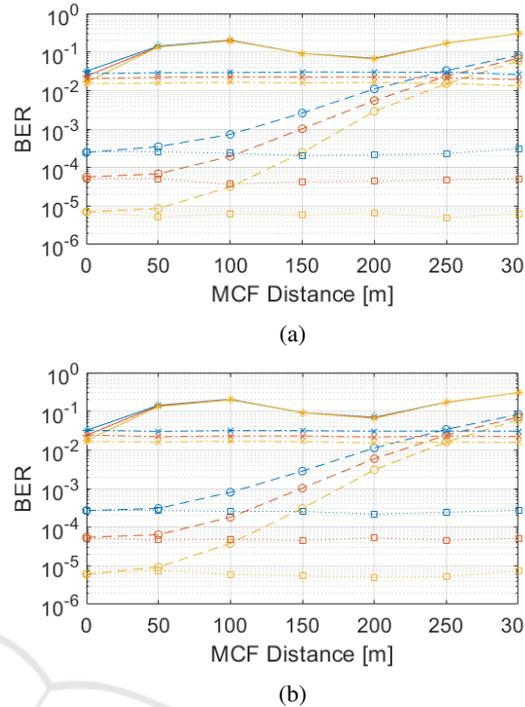
Figure 9: BER as a function of the MCF length, before SSBI removal with dispersion (continuous line) and without dispersion (dashed and dotted line), and after SSBI removal with dispersion (dashed line) and without dispersion (dotted line), for a laser linewidth of: (a) 100 kHz and (b) 5 MHz.
