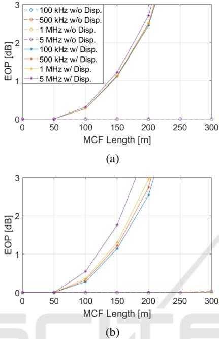
Figure 4: EOP as a function of the MCF length for different laser linewidths, with and without dispersion, for: (a) a walk-off of 1 ns/20 km and (b) a walk-off of 10 ns/20 km.
