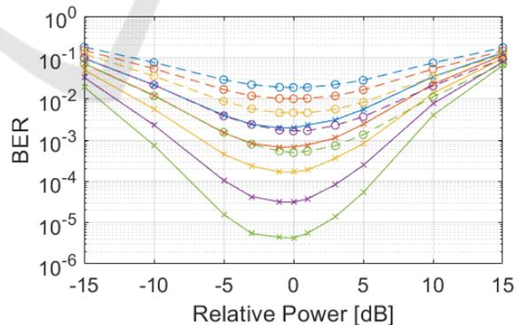
Figure 5: BER as a function of the relative power before (continuous line) and after (dashed line) SSBI removal for a SNR of: 12 (blue), 13 (red), 14 (yellow), 15 (purple) and 16 (green) dB.
