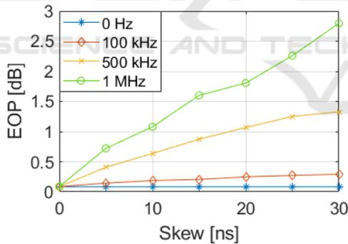
Figure 2: EOP as a function of the skew, for different laser linewidths.
