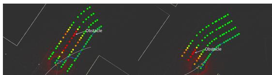
Figure 9: Vehicle trajectory at different frames during static obstacle avoidance, showing the waypoint plan (blue line) and the pure pursuit trajectory (white arc).
