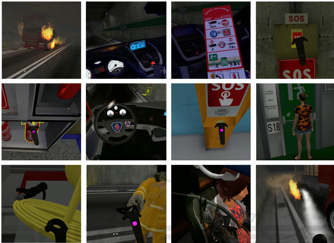
Figure 5: Road tunnel fire (first picture) and some of the available interactions: hazard lights, safety brochure, SOS button, extinguisher, vehicle engine, SOS telephone, SOS shelter doors, fire hose, NPC firefighter, scissors, and handline nozzle.
