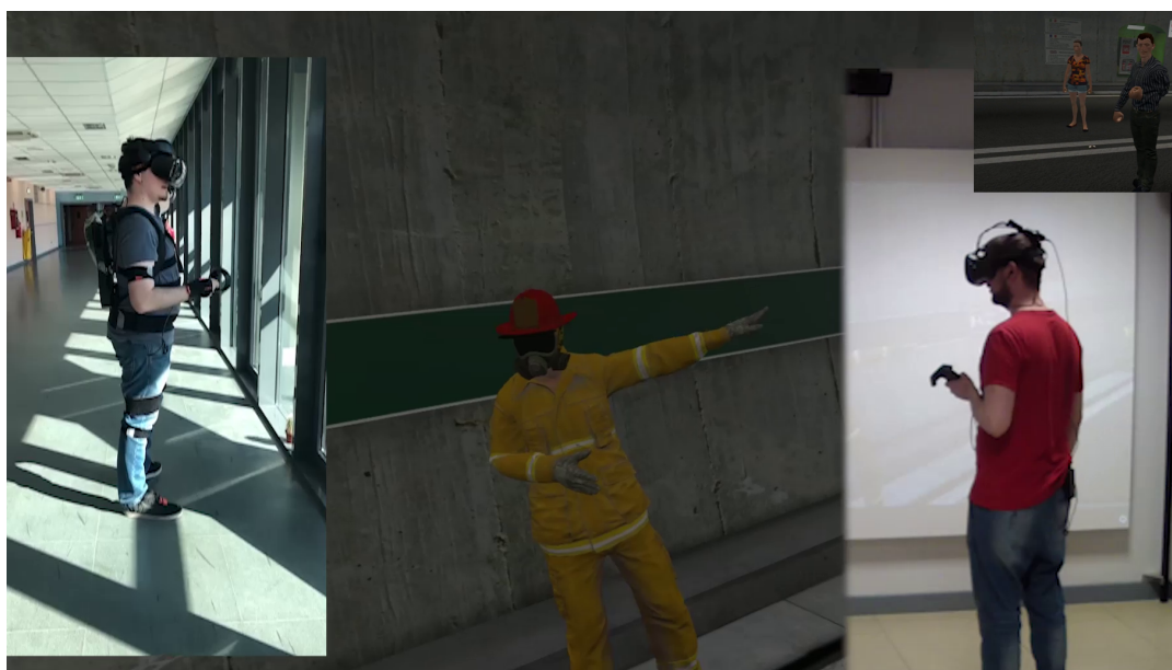
Figure 4: Combined use of different devices and technologies in a multi-user FrèjusVR session. On the left: User 1, playing as a firefighter, equipped with an inside-out VR HMD, a backpack PC and a motion capture suit. On the top right: Point-Of-View (POV) of User 1, viewing User 2 and User 3. On the right: User 2, playing as a car driver, equipped with an outside-in VR HMD. In the center: POV of User 2, viewing User 1. User 3 playing as a truck driver from a desktop PC (not shown).
