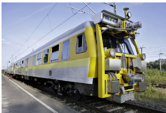
Figure 1: Measurement train “Limez III” (Wirth, 2008).
