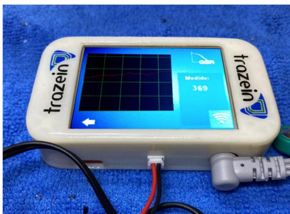
Figure 9: Trazein HMI showing GSR signal real-time acquisition with Subject 2.
