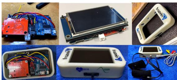
Figure 5: Final 3D printed manufactured device.
