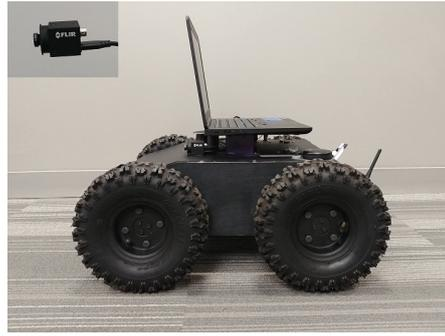
Figure 1: Dr. Robot Jaguar mobile robot platform with FLIR Blackfly S camera onboard.
