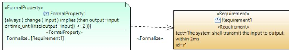
Figure 1: Example of a FormalProperty formalizing a requirement.
