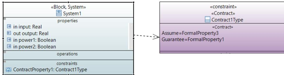
Figure 2: Example of a component contract.
