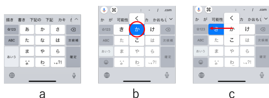
Figure 3: A typical input flow for a Japanese flick keyboard (which is available on iOS).
