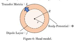
A dipole layer was virtually placed in the brain of this head model. On this layer, multiple dipole signal sources in the radiation direction were installed at equal intervals. The signal sources generated in the brain can be equivalently represented by dipoles on this layer, regardless of the number or direction. Using the transfer matrix L from this dipole layer to the scalp surface, the process of observing the scalp surface potential  $\Phi$  was modeled by the following equation.
