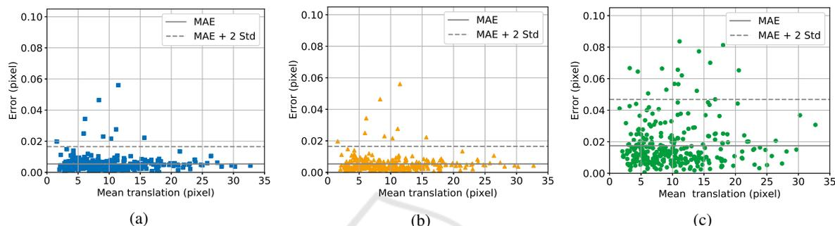
Figure 6: Visualization of the pixel error versus mean translation for (a) MM, (b) combination algorithm and (c) IP.
