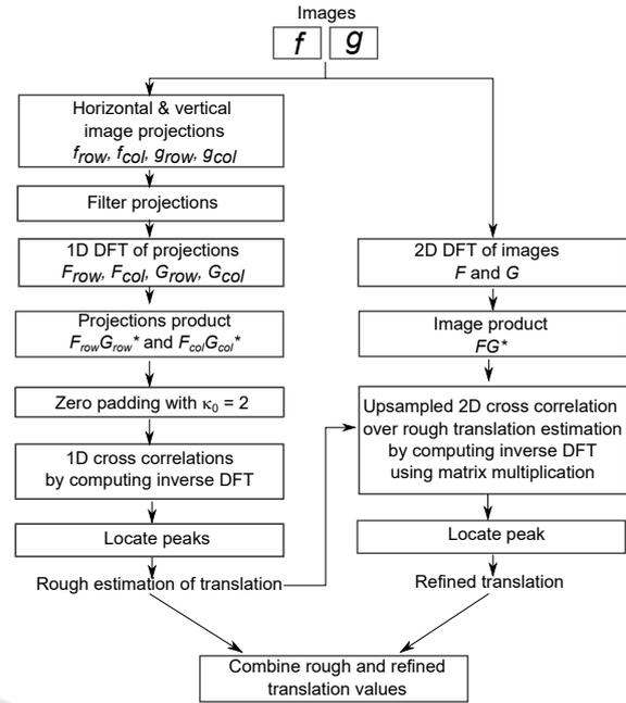
Figure 1: Computational process of the proposed combination approach.
