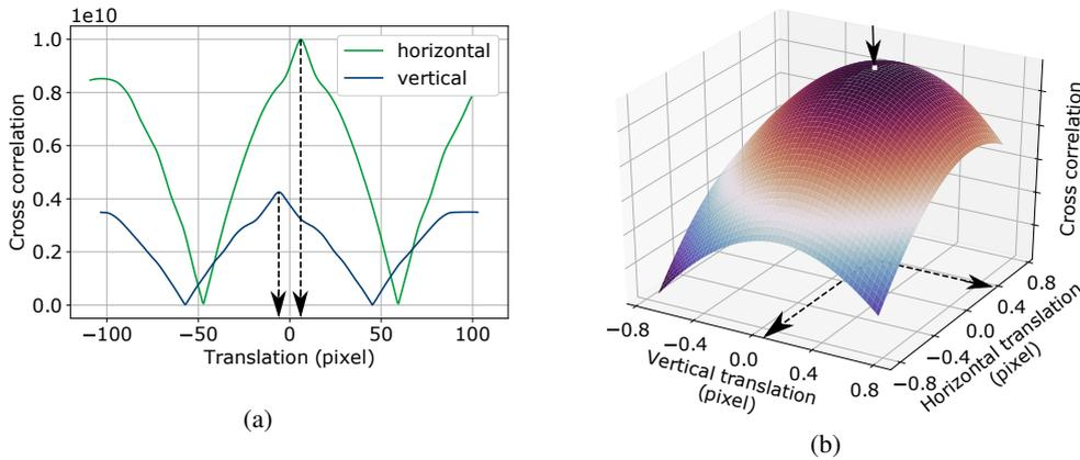
Figure 3: Visualization for the main steps of combination algorithm: (a) 1D rough cross correlations and (b) 2D refined cross correlation around the rough estimation, where the locations of peaks are marked by arrows.
