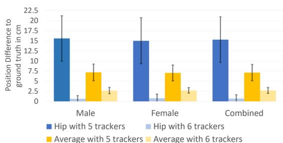
Figure 3: Position difference between ground truth and simulated results for walking animations with and without a hip target.
