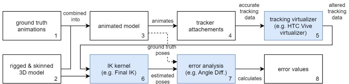
Figure 2: Data flow of the simulation process. The blue highlighted components offer interfaces for developing custom implementations.
