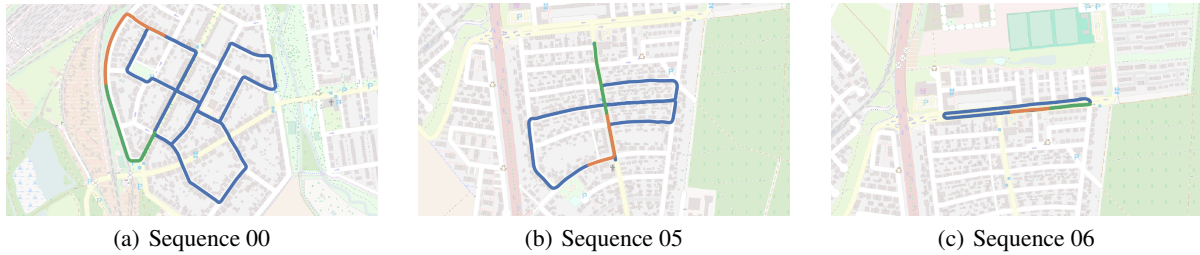
Figure 4: Illustration of the training (blue), validation (orange), and test (green) splits on the three KITTI-VO sequences we are using. Map data copyrighted (OpenStreetMap contributors, 2017) and available from https://www.openstreetmap.org .
