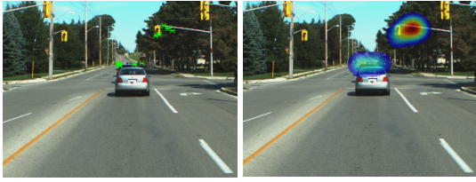
Figure 2: An example of PoG and matching fixation saliency map. (left): PoGs projected onto the forward stereo system of the vehicle obtained with the preceding 15 consecutive frames. (right): The driver’s point of gaze as a 2-D Gaussian distribution.
