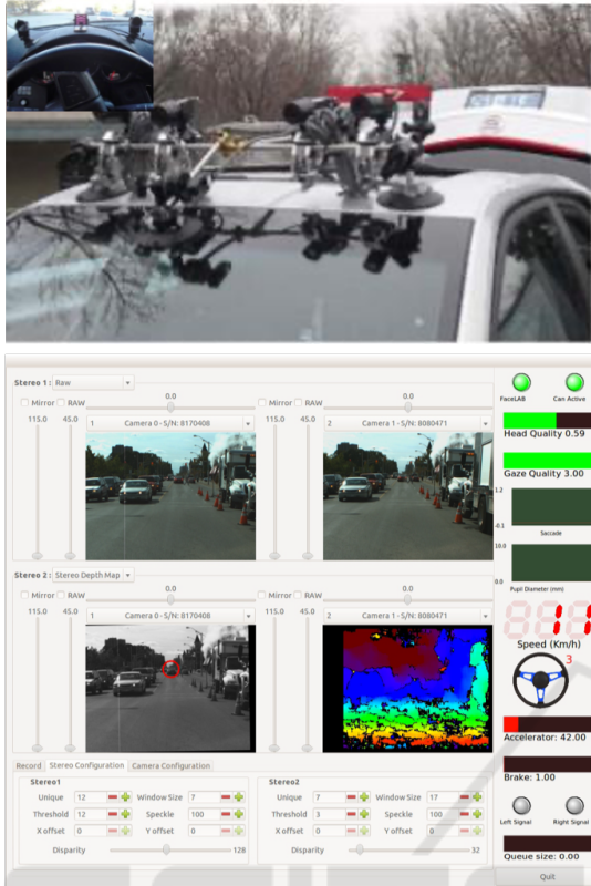
Figure 1: RoadLAB configuration. (top): vehicular configuration: stereoscopic vision system on rooftop and 3D infrared eye-tracker located on the dashboard. (bottom): software systems: The on-board system displays frame sequences with depth maps, dynamic vehicle features, and eye-tracker data.
