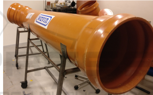
Figure 2: An example pipe configuration, used for collecting the point cloud data from the physical setup.
