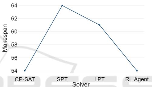
(d) SAC evaluation: RL agent has found a solution with the shortest makespan
