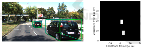
Figure 3: Vehicle Localisation in bird's-eye view: The left image shows the 3D bounding box output and the right image shows the tight bounding boxes for the cars we obtain in bird's-eye view in camera frame in metric scale from the procedure described in Sec. 3.1.3. The camera center for the right image is at (0,0) of XZ plane facing towards positive Z axis.
