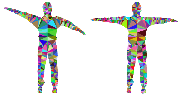
Figure 5: Triangulation result of the Constrained Delaunay algorithm using the simplified mask contour as constraints and the aligned limb model with n = 5 interpolated interim points per limb (left). Resulting mesh after deformation of triangulation result using the interpolated reference model's skeleton points as moving anchors for the ARAP transformation algorithm (right).
