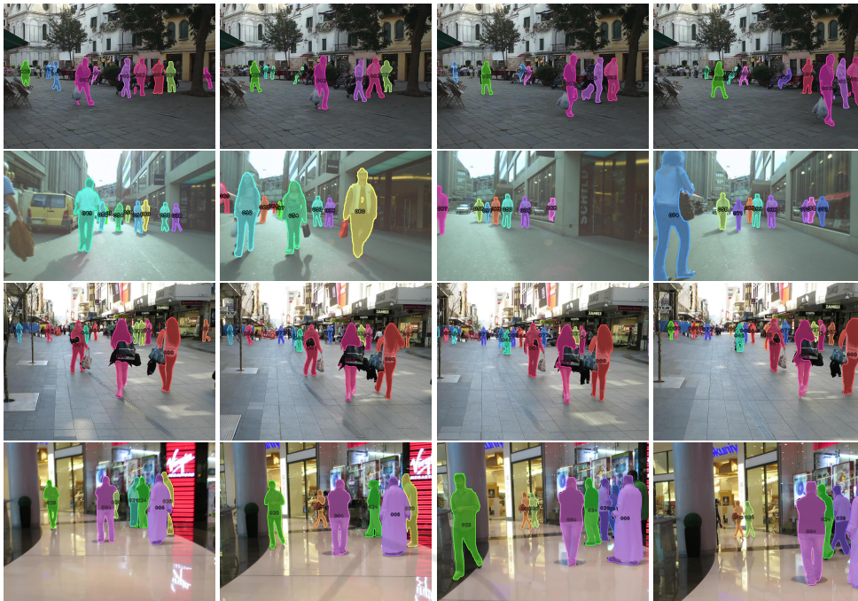
Figure 5: Examples of images from the MOTs test set, with segmentation tracks by SORTS+RReID. Images are taken 30 frames apart. Best viewed in color, preferably on a screen.
